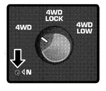
**NOTE:** The 4x4 system will not allow shifts between 4WD/4WD LOCK if the rear wheels are spinning (no traction). In this situation, a position indicator light will flash and the original position indicator light will remain on. At this time, reduce speed and stop spinning the
